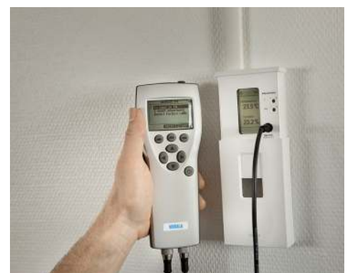
On-site calibration with HM70 Handheld Meter
