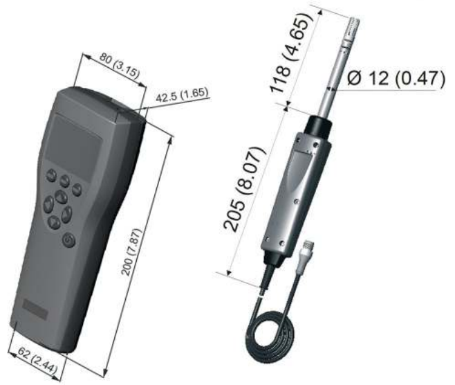
MI70 indicator and HMP75 probe dimensions in mm (inches)
